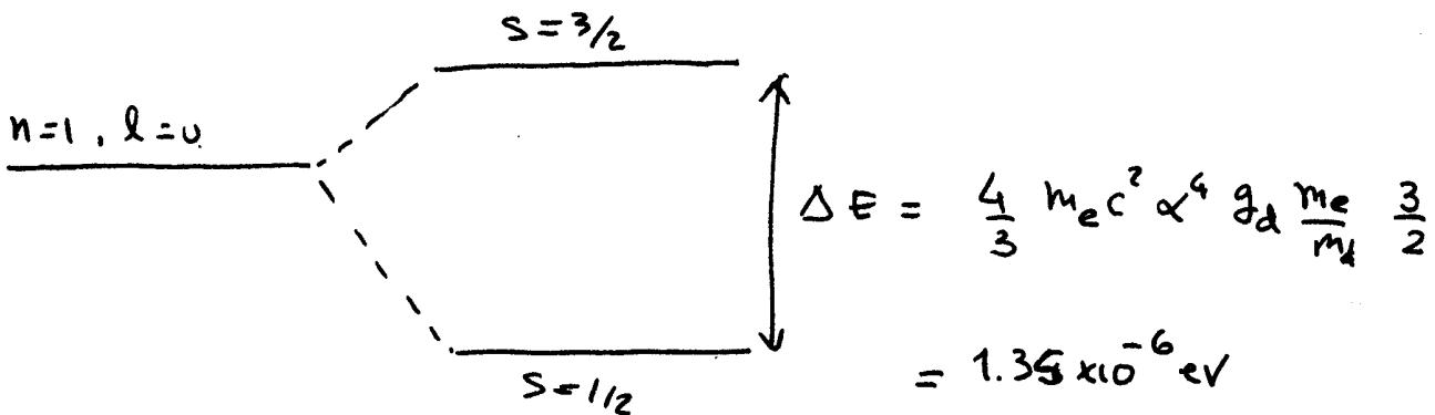
$$\lambda = \frac{c}{f} = \frac{hc}{\Delta E} = \frac{1240 \times 10^{-7} \text{ cm} \cdot \text{eV}}{1.35 \times 10^{-6} \text{ eV}} = 91.8 \text{ cm}$$
