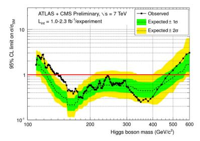
**Fig. 21.** Combined results of the ATLAS and CMS Collaborations presented at the Hadron Collider Workshop in November 2011. The solid line is the experimental upper bound, at 95% confidence level, on the cross section for Higgs boson production divided by the cross section of the Standard Model. The dashed line is the expected 95% exclusion bound, and the green and yellow bands are the one- and two-standard deviation bands around that expected bound.
