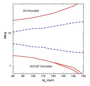
**Fig. 17.** Current Tevatron bounds on the mass  $M_H$  of the charged Higgs as a function of  $\tan \beta$ . The small sliver near the lower-right corner is excluded by CDF but not by D0. The dashed lines are the bounds which are projected for the ATLAS experiment with 30 fb<sup>-1</sup> of data; the regions that would then be excluded are those outside the dashed lines.
